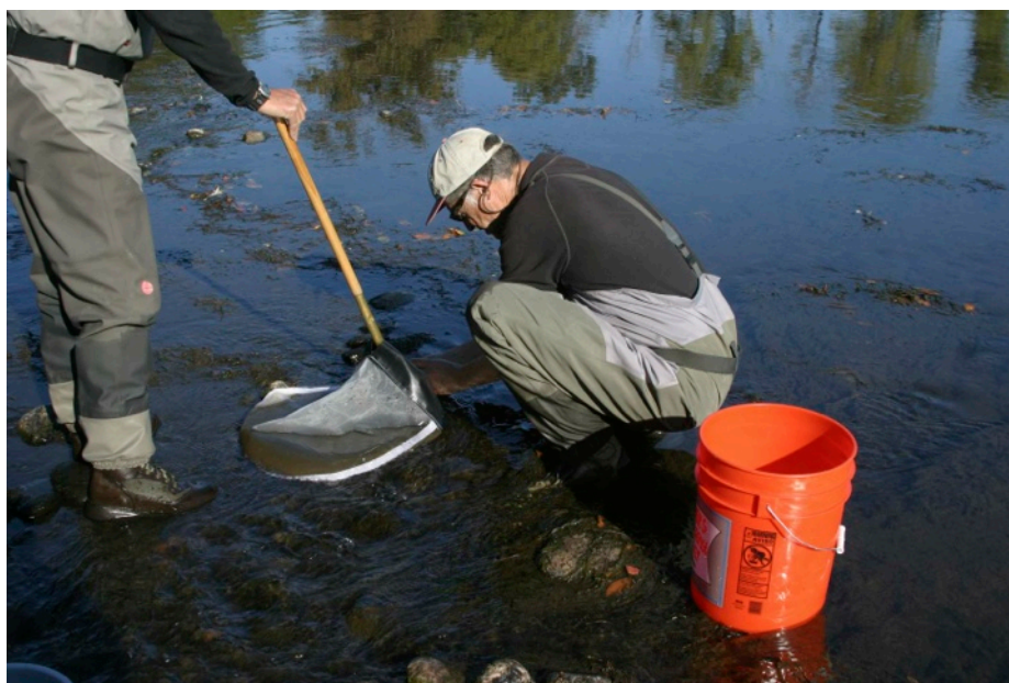
Figure 3. Collecting macroinvertebrate sample with D-frame kick net.
