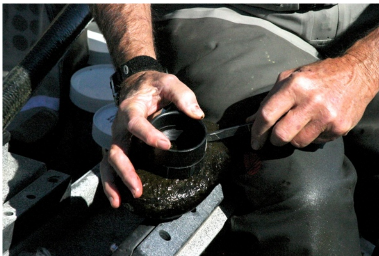
Figure 2. Plastic pipe end used to define algal sampling area.
